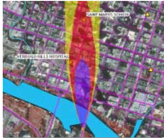
The toxic plume generated by SAFER Systems software is superimposed onto the GIS map
