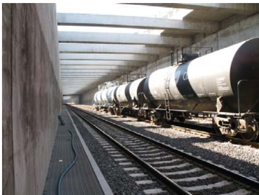
Chlorine tank cars in the trench during the ACTA simulation of a potential terrorist event leading to an opened or damaged valve on one of the cars.
